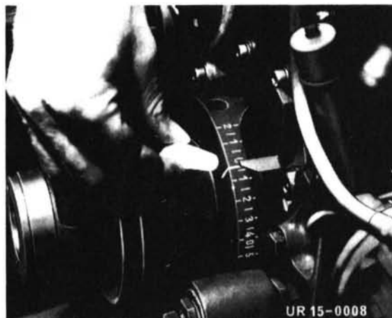
Figure 45 Mark firing point 2^{\circ} bTDC at basic setting 404.1
