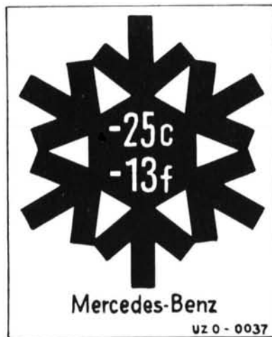
Figure 31 Antifreeze filling to -25^{\circ}\text{C} or -13^{\circ}\text{F}
